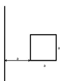
Infinite wire is located next to a loop. Loop is given current, which changes with respect to time. The rate is given by dI/dt.
